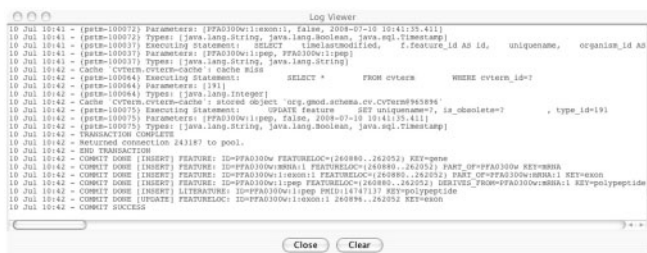
Fig. 7. Snapshot of the Artemis log viewer, using log4j to generate log messages and errors. It records SQL statements and can be used to monitor changes to the database. The last seven lines in this log are generated to show the changes made to the database in a more human readable format.
