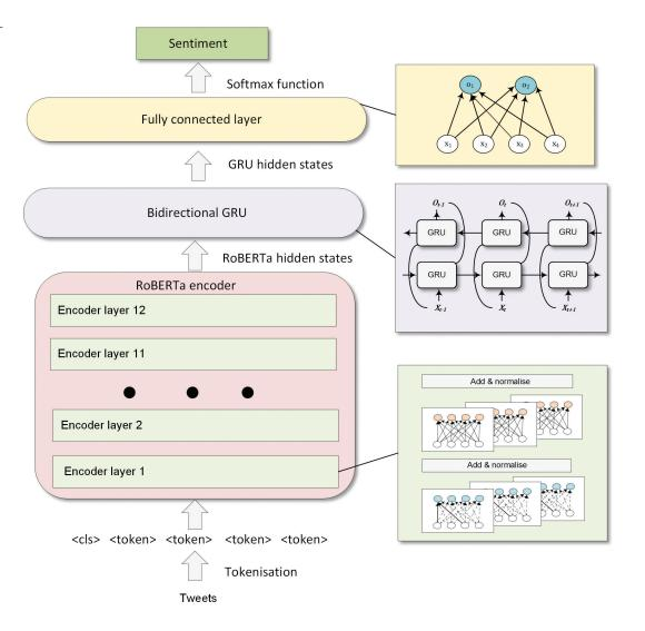
multiple self-attention heads to obtain 768 tweets' hidden representations. The tweets' hidden representations can then be allocated to sentiment classes through a bidirectional GRU and fully connected layer.
