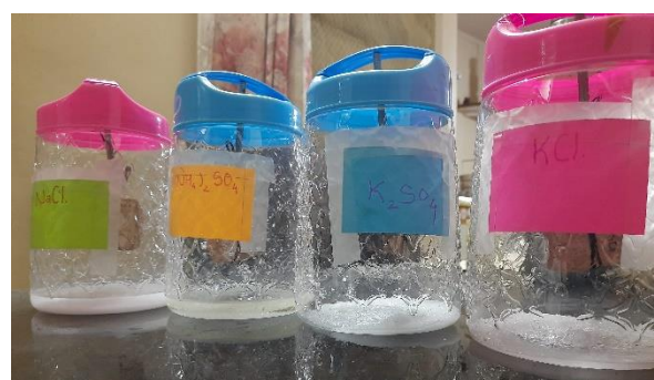
Figure 8 Lime plaster samples used for experiment Figure 7 Jars containing different salt solutions
