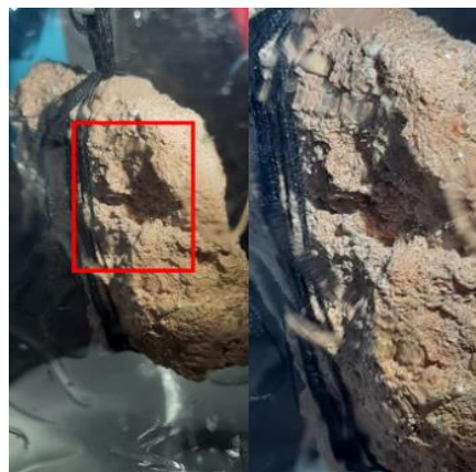
Figure 23 Mold growth observed under 96% relative humidity
