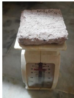
Figure 8 Lime plaster samples used for experiment Figure 7 Jars containing different salt solutions
