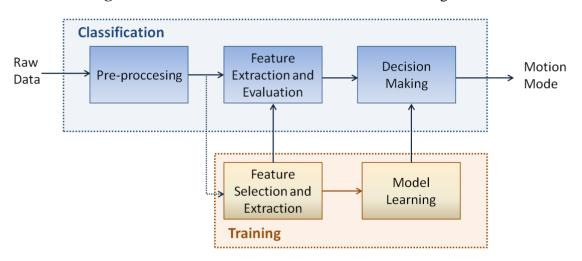
Figure 1. Scheme of a classifier for motion mode recognition.
