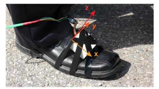
Figure 10. IMU attached on the foot and used as a reference for step detection assessment.
