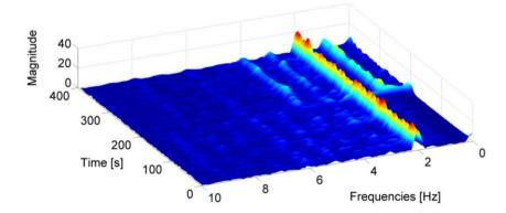
In order to better analyse how these frequency peaks change over time, the three main frequencies, obtained by evaluating the first three maxima in the spectrogram, are reported over time. The estimated three dominant frequencies for a pedestrian test are reported in Figure 5 and are now further analysed.
