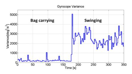
**Figure 3.** Variance of the gyroscope signal (norm) for IMU in the swinging hand and IMU in the user's bag.
