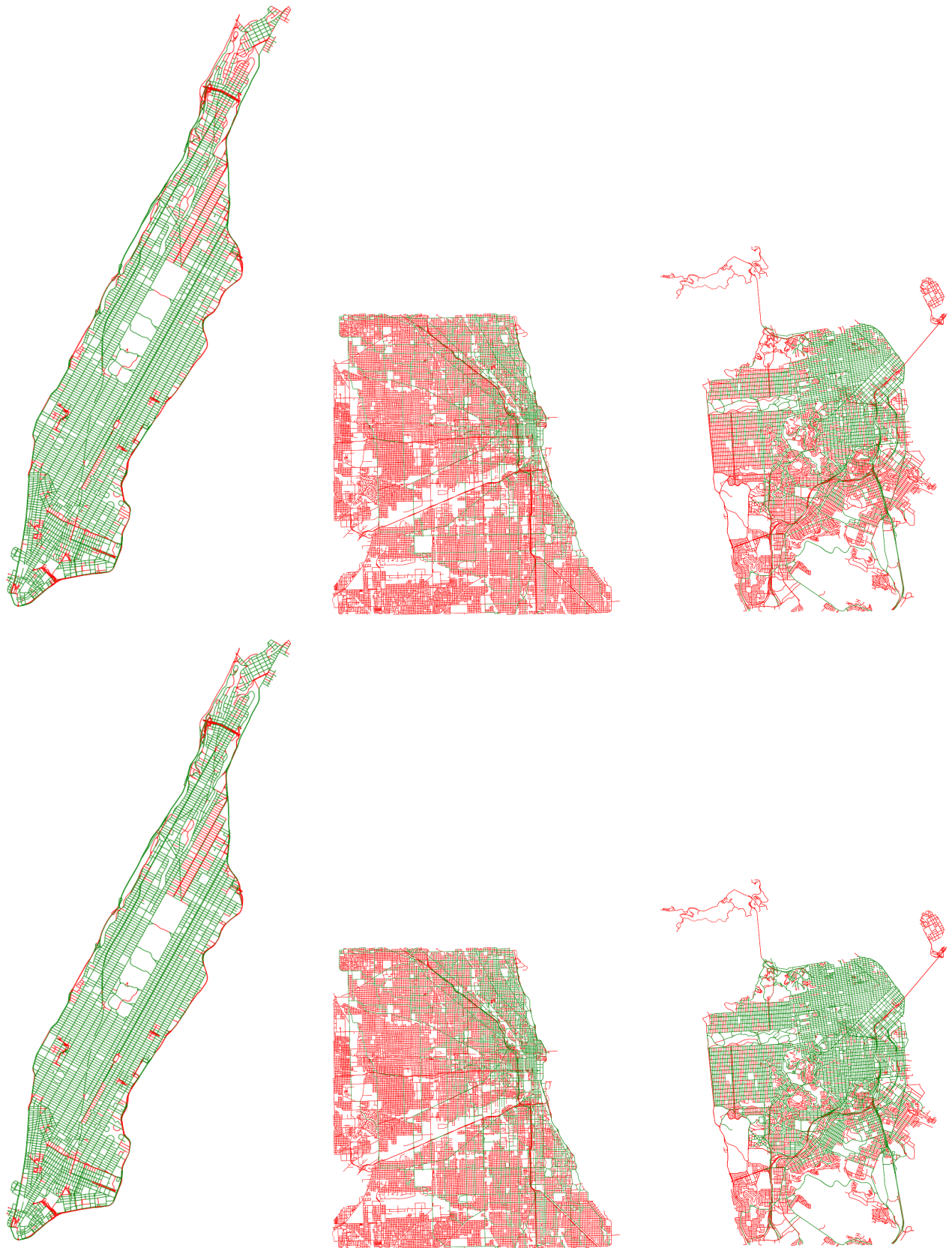
Fig. S18. Spatial coverage at different saturation levels. NYC, Chicago, and San Francisco are shown in the first, second, and third columns. The top row shows the coverage when N_T = 10\% , and the bottom row shows the coverage when N_T = 75\% of trips. Covered segments are colored green, while uncovered segments are colored red. As can be seen when N_T is small (top row), predominantly segments in the city center are covered. When N_T increases, areas outside of the city center become covered. See "Spatial bias of drive-by sensing" section.
