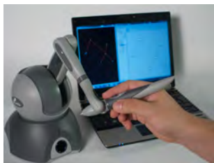
Figure 4: Interacting with the spatial haptic view using the stylus of a PHANTOM Omni haptic device.
